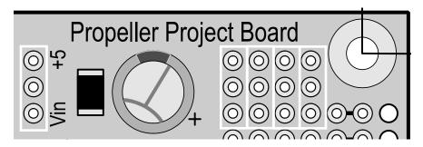
**Note:** If only video or PS/2 peripherals are needed for an application, standard connectors may be used on the Propeller Proto Board. If only PS/2 connectors are installed, only the 100  $\Omega$  resistors need to be installed. If only a VGA connector is installed, only the 470  $\Omega$  resistors need to be installed.
