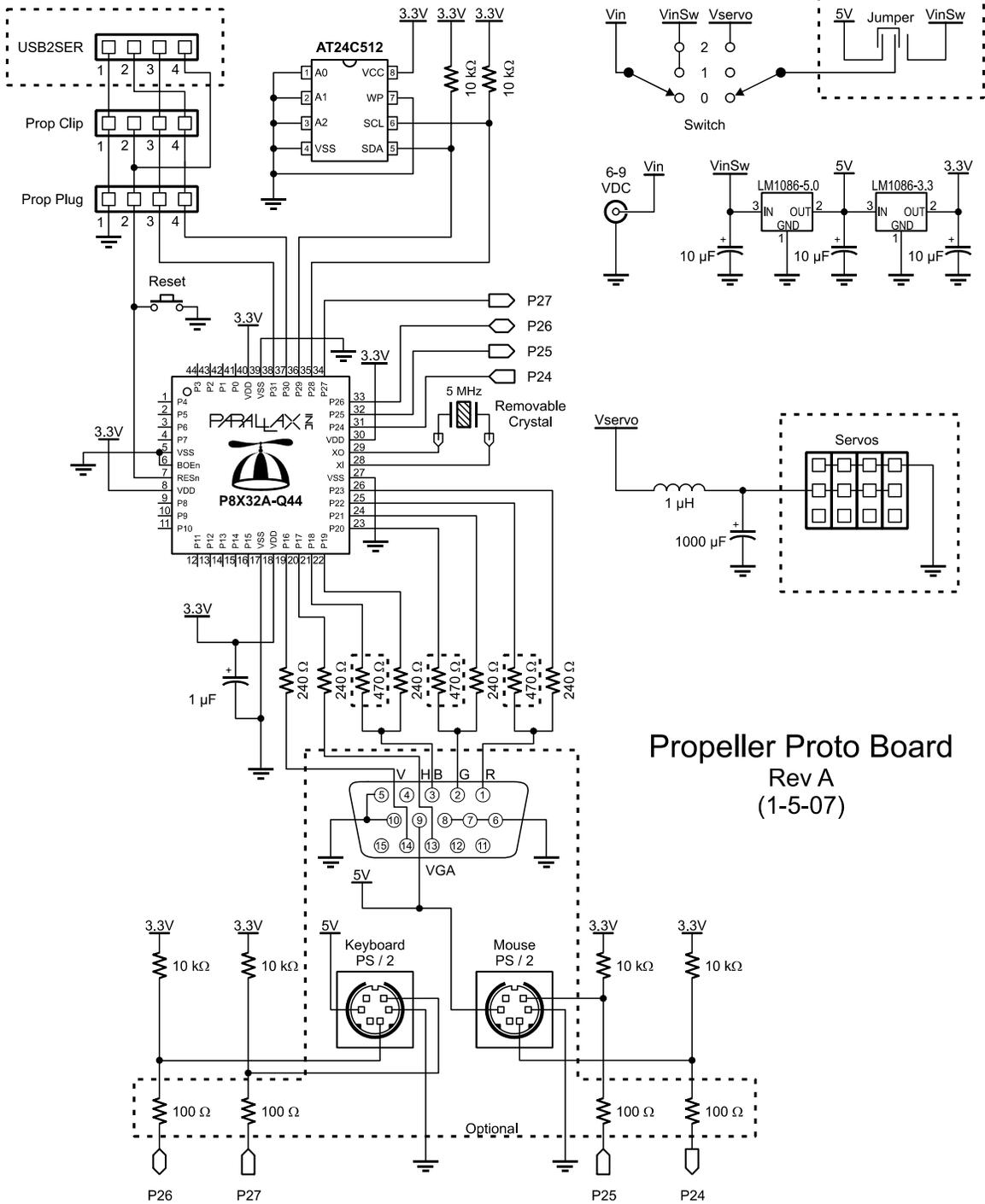
Propeller Proto Board
